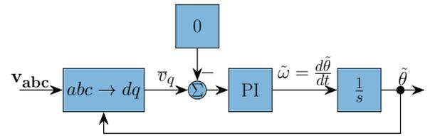
Fig. 2: Three-phase synchronous reference frame PLL
