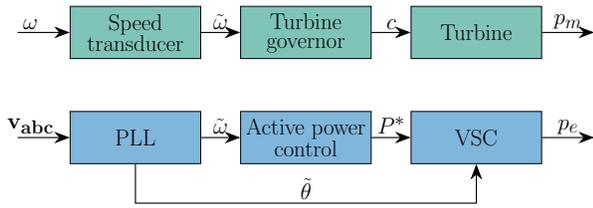
Fig. 1: Analogy between synchronous generators and grid-following VSCs
