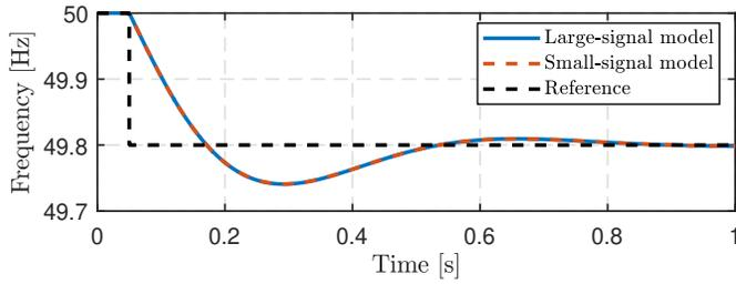
Fig. 3: Validation of the small-signal SRF PLL model
