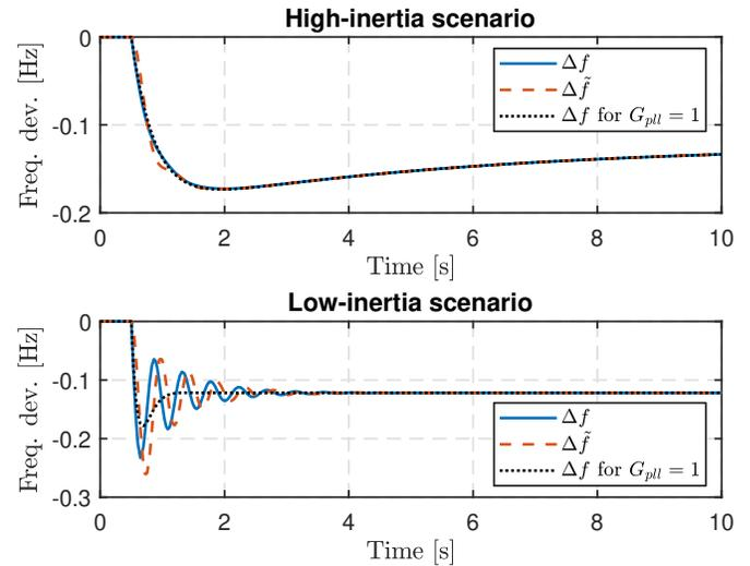
Fig. 5: Impact of PLL dynamics on grid frequency
