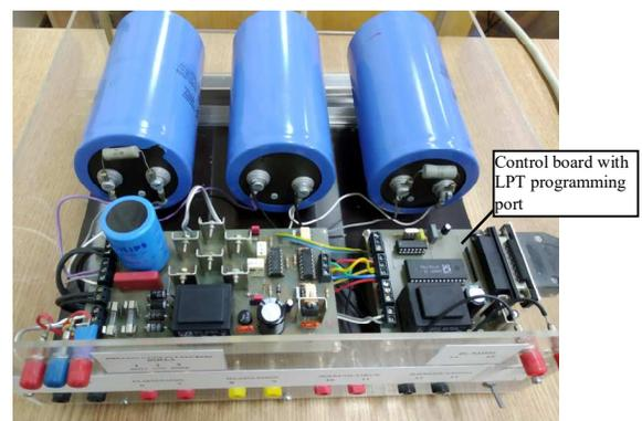
Fig. 2. Single-phase 1 kW half-bridge VSI
